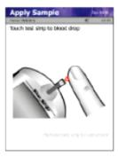
**Caution:** Keep the meter flat or pointing downward while applying sample and during testing to prevent sample from seeping into the test strip insert slot.
