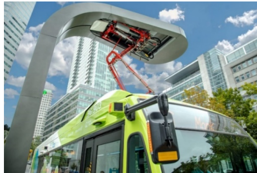
An overhead OppCharge fast charger. Source: inside EVs.
