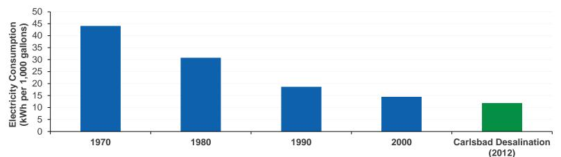
New RO membrane configurations minimize energy consumption and reduce system size and cost
