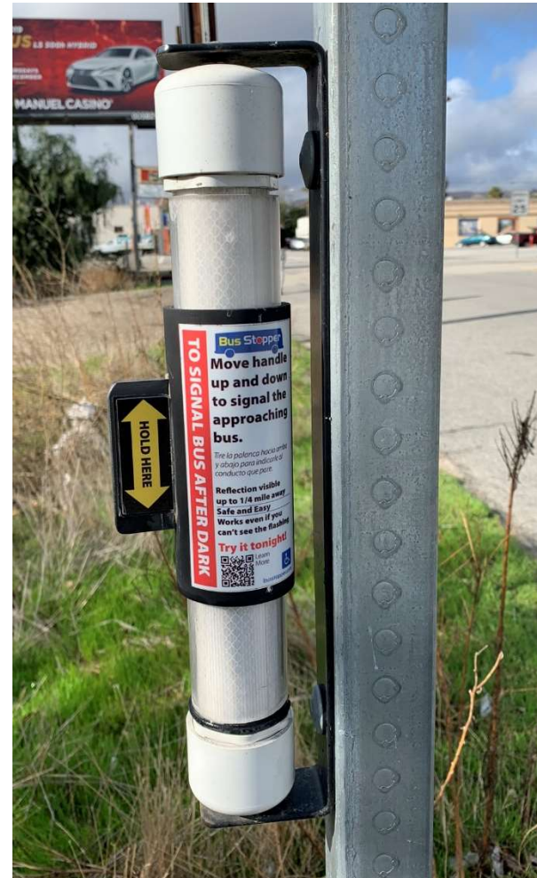
The bus stop on Los Angeles Avenue near Nardo Street includes a mechanism to signal buses after dark. Many stops lack lights.
