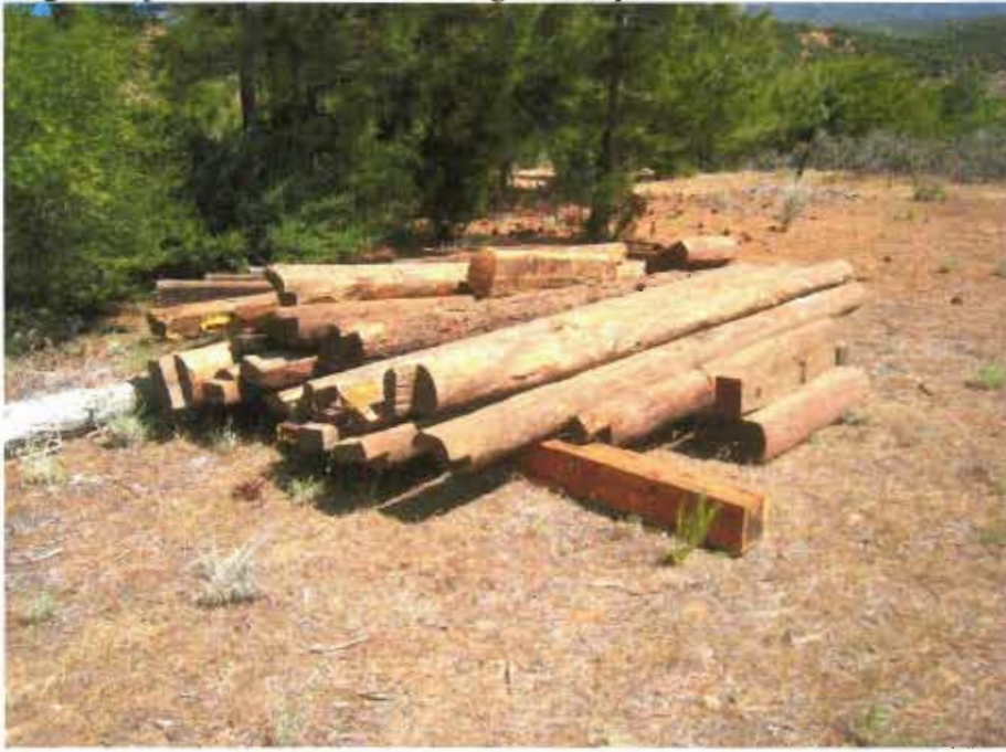
Log floor joists saved for use in log wall repair
