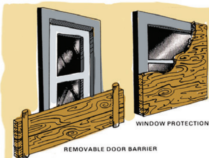
Figure 14: Typical Window/Door Protection – Use of plywood or timbers can help protect windows and doors from damage.
