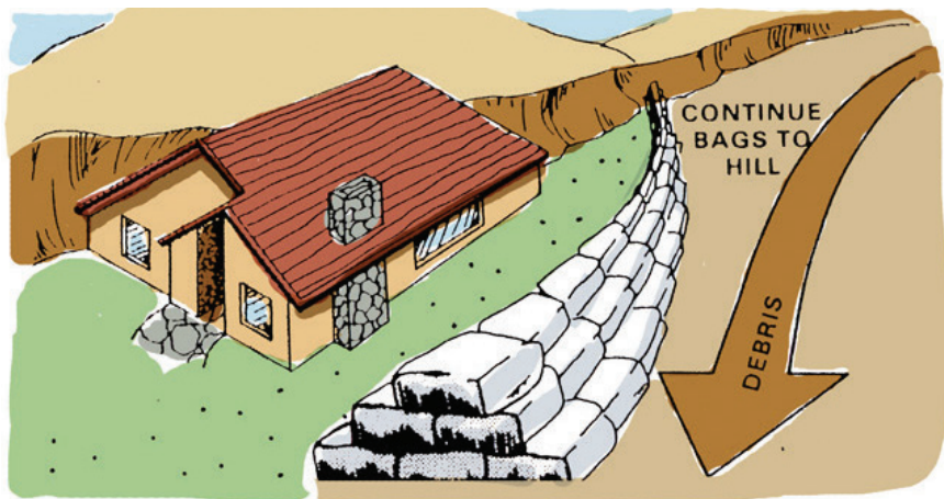
Figure 7: Directing Debris Flows – The use of a sandbag wall to deflect debris away from structures.
